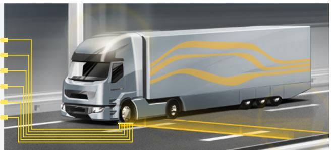
WIM reliably determines and checks axle weights, gross weight and trailer weight.
