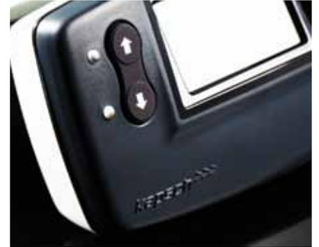
The Kapsch OBU (on-board unit) TS3290/00A is the in-vehicle part of the Kapsch Satellite Tolling System which facilitates the implementation of road user charging schemes based on geographical positions obtained from a GNSS (Global Navigation Satellite System).
