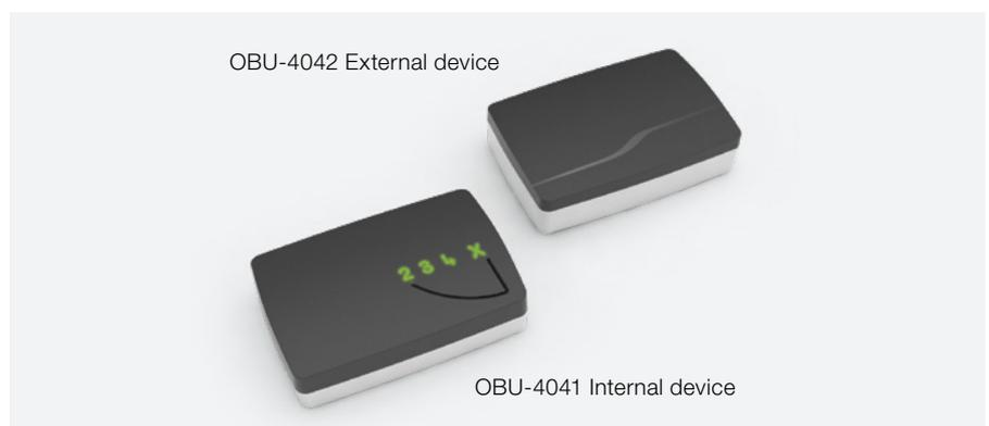
The two devices are mounted to the windscreen opposite of each other by using adhesive. Communication between the units takes place through the windscreen by means of a proprietary light link.
