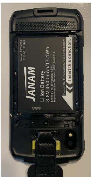
Figure 14 Battery Placement
