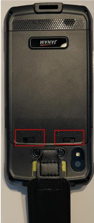
Figure 13 Janam XT30 Display Unit Battery Tabs
