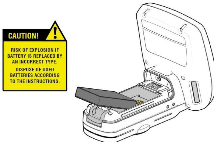
Figure 7 Trigger Unit Battery Placement
